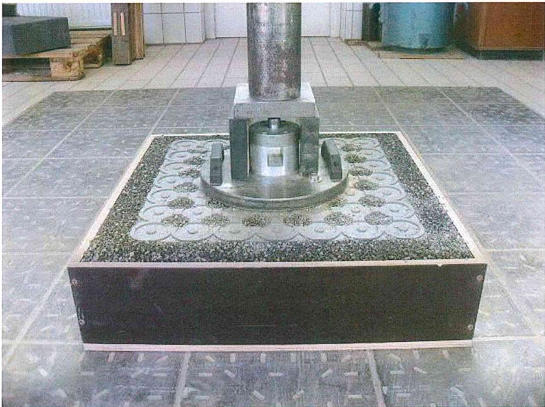
Figure 1: Test setup – "Cellular slabs Horses Home" on an artificially manufactured subgrade
